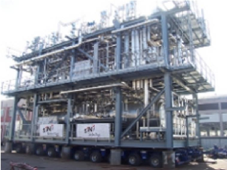
**March, 2006 - Vietnam:** JGC Corporation selects Siirtec Nigi as the supplier of technology, basic design, detailed engineering, material and erection of a sulphur recovery plant for Dung Quat refinery, the first refinery project in Vietnam launched by Petrovietnam - Vietnam Oil and Gas Corporation. The Modular SRU, with a capacity of 5 tpd, is designed to recover more than 95% of sulphur with 99.9 + % of purity.
